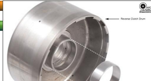
Bushing failure and/or reverse clutch drum journal damage
